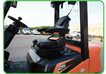
New Mechanical Vibration-Damping Seat.
