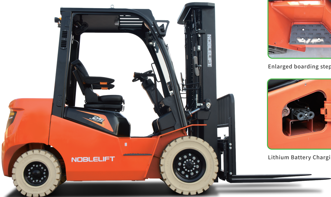
The use of a smaller diameter steering wheel reduces the fatigue for the operator.
