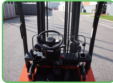
The widened mast offers better visibility.
