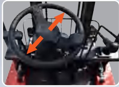
A smaller diameter steering wheel is used to reduce operator fatigue.
