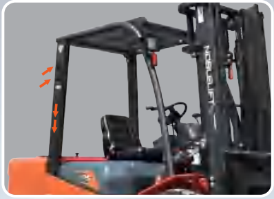
The engine intake pipe uses a high-mounted independent intake, effectively preventing dust from entering.
