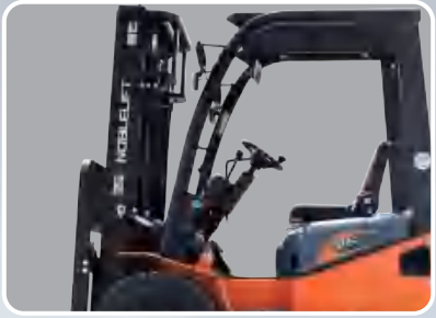
Increase the leg and headroom for the driver, and enhance visibility for operation.
